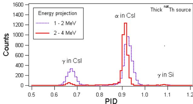
Figure 2b: Projection of Fig. 2a data on the PID axis for two energy ranges.
