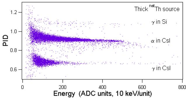
Figure 2a: PID versus energy for alphas and gammas in CsI(Tl) and from gammas in photodiode.
