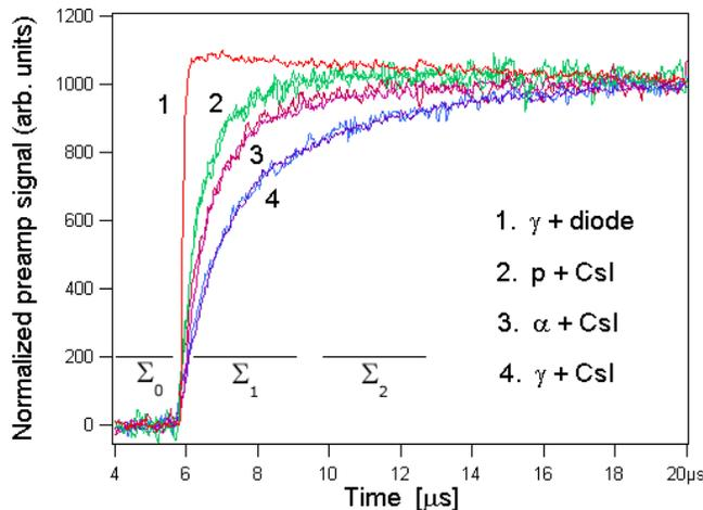
Figure 1: Normalized pulses from CsI(Tl) + photodiode output from the charge integrating preamplifier.
