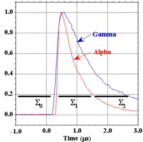
Figure 3: Normalized alpha and gamma pulses from CsI(Tl) + PMT output directly into Polaris spectrometer.
